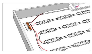
Wire both ends of LED modules to the power supply (refer to page 2). For multiple series, connect them in parallel to avoid voltage drop and ensure even brightness.
