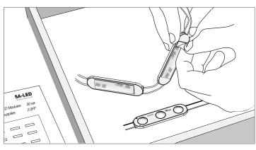
Remove the tape from the back of the LEDs and stick them in place according to the provided LED layout, including the appropriate module pitch (refer to Figure 1 on page 2).
